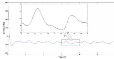
Fig. 3. Torque with 0.5 tip speed ratio
