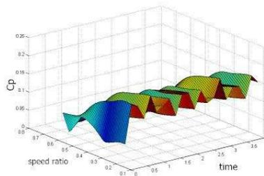
Fig. 4. Torque coefficient with 8.5m/s wind
