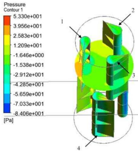
Fig. 6. Pressure distribution of wind speed is 8.5m/s
