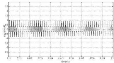
Fig. 17. Stator current of the d-axis of an enlarged curve
