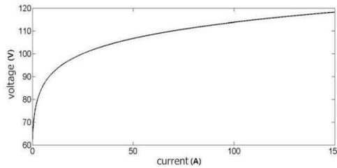
Fig. 9. Curves of voltage and current in electrolysis cell
