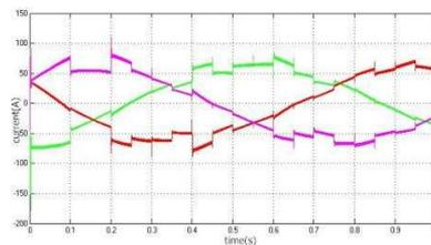
Fig. 18. Three phase current variation curve of generator
