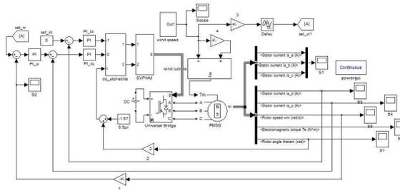
Fig. 8. Power generation system simulation model
