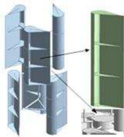
Fig. 2. 3D model of Senegal type wind turbine
